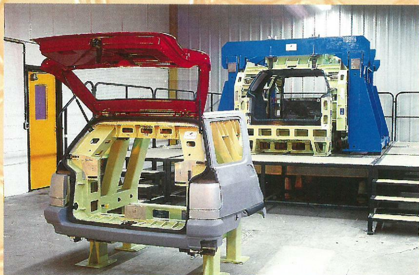
Interior and exterior presentation models (MAPI, MAPEX) were used to ensure optimum quality in the assembly of the ZX.
